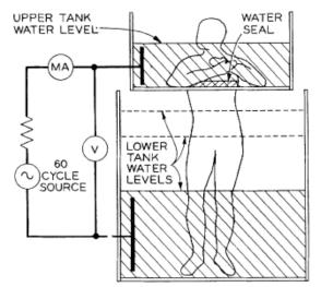
Figure 2. Electric field measurements
