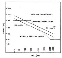
Figure 4.2 Fibrillating Current Versus Shock Duration (Dalziel, C. F., 1968)
