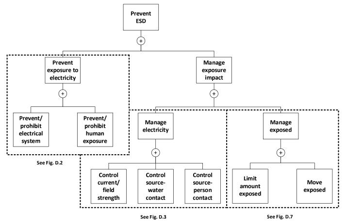
Figure D.1 Top Level of ESD Concept Tree with Selected Lower-Tiered Gates.
