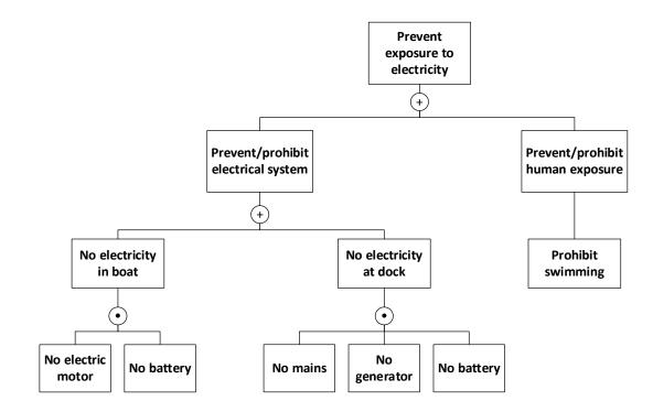
Figure D.2 Prevent Exposure Branch of ESDCT.
