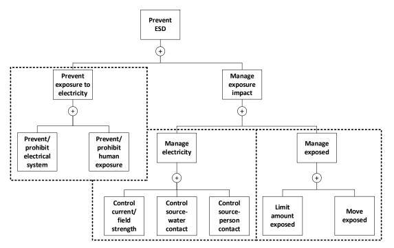
Figure 3.15 Top Level of ESD Concept Tree with Selected Lower-Tiered Gates.
