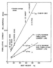
Figure 4.1 Fibrillating Current versus Body Weight for Various Animals for a 3-second Duration Shock (Dalziel, C. F., 1968)
