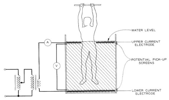
Figure 3. Electric field measurement; loss of muscular control
