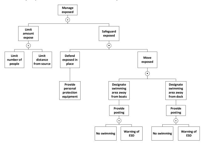
Figure 3.18 Manage Exposed Branch of ESDCT.
