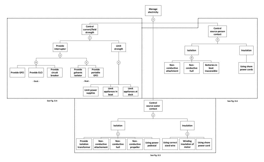
Figure D.3 Manage Electricity Branch of ESDCT with Selected Lower-Tiered Gates
