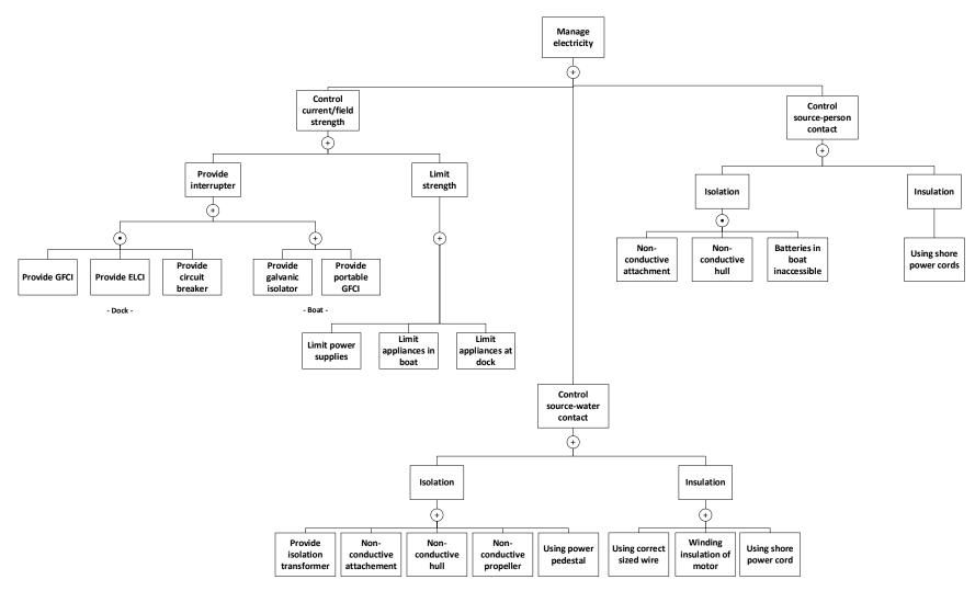
Figure 3.17 Manage Electricity Branch of ESDCT.
