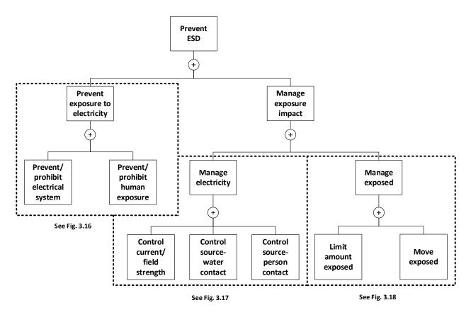
Figure 3.15 Top Level of ESD Concept Tree with Selected Lower-Tiered Gates.
