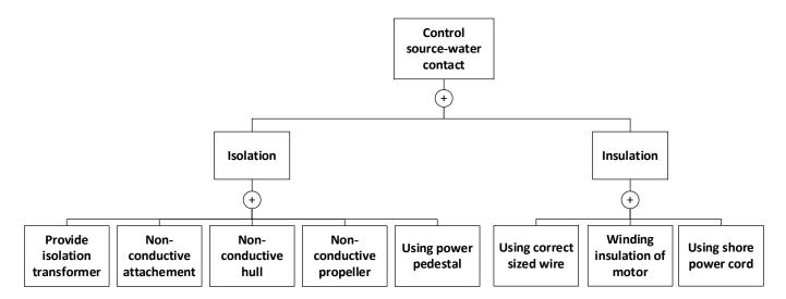
Figure D.5 Control Source–Water Contact Branch of ESDCT.
