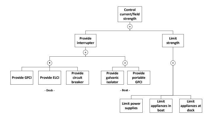
Figure D.4 Control Current/Field Strength Branch of ESDCT.
